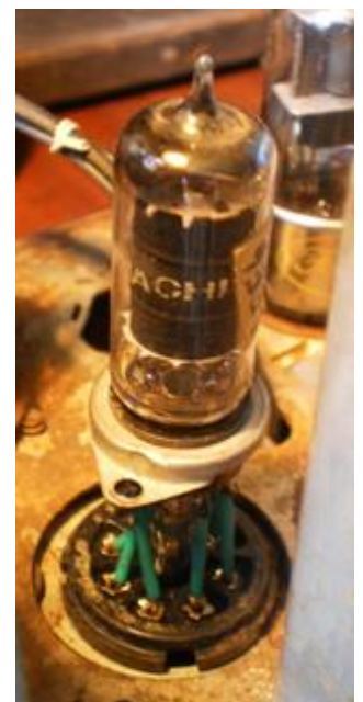
Left the original scheme of valves and right exotic 6BE6 valve connected with an adaptation by wires to the base of the original 6SA7.
