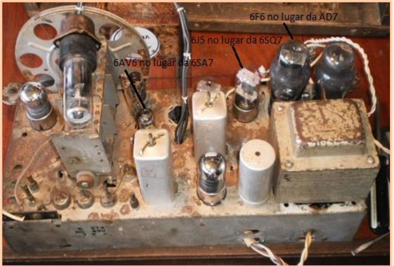
The chassis as received with non-original valves.
